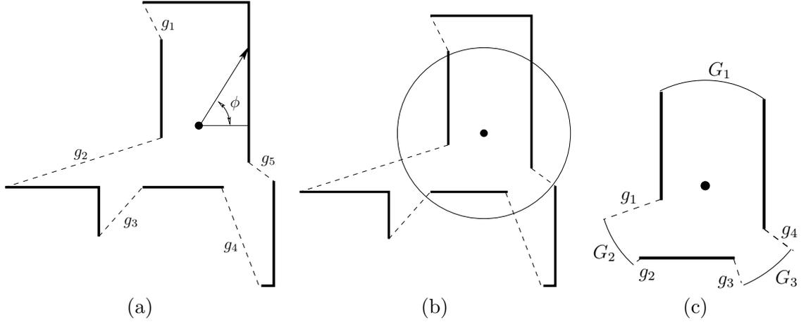
Figure 10: Gap sensor models: (a) Five discontinuities in depth are observed. (b) A limited range is considered. (c) Two kinds of gaps are obtained for limited range.
