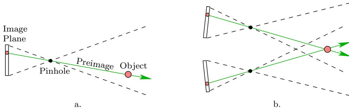
Figure 16: a) Using the pinhole camera model, the preimage of a point object is an infinite ray that connects from the pinhole to the object. b) From matching the same object in two camera images, its location can be determined by intersecting the two preimage rays.
