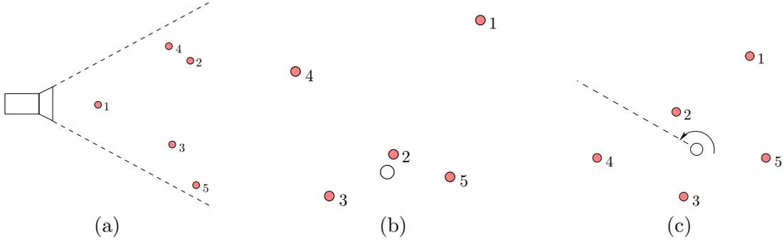
Figure 9: Three kinds of compound relational sensors: (a) The linear sensor observes that the landmarks are ordered from left to right as (4, 2, 1, 3, 5). (b) This sensor sorts the landmarks closest to farthest, resulting in the observation (2, 3, 5, 4, 1). (c) The cyclic sensor sweeps counterclockwise and yields the cyclic ordering (1, 2, 4, 3, 5)
