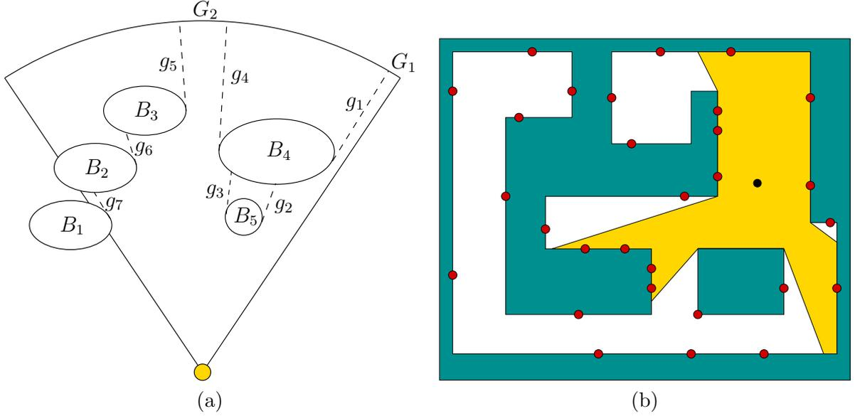
Figure 11: (a) A gap sensor among multiple bodies. (b) A sensor that counts landmarks between gaps.
