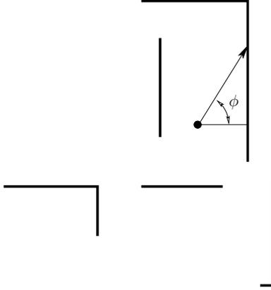
Figure 7: For the omnidirectional depth sensor, Model 12 a function  $y : S^1 \rightarrow [0, \infty)$  is obtained in which each  $y(\phi)$  is the depth in the direction  $\theta + \phi$ . The figure shows how the depth data appears for the environment in Figure 6(a) and  $\theta = 0$ .
