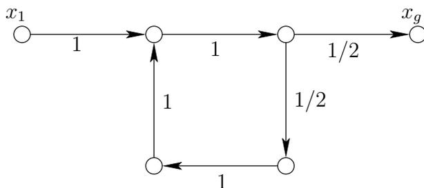
Figure 3: Probabilistic uncertainty can cause value iteration to converge only in the limit. Edges are labeled with transition probabilities. In this example, nature can cause executions of arbitrary length. However, executions that traverse the cycle in the graph many times are unlikely. Assuming the cost of each transition is 1, the cost-to-go for  $x_1$  converges  $2 + 4 \sum_{i=0}^{\infty} i \left(\frac{1}{2}\right)^{i+1} + 1 = 7$ .
