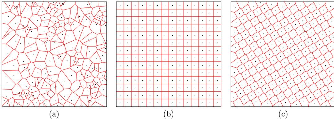
Figure 4: Three ways to select samples in the unit square. Dots represent samples, the lines show their respective Voronoi cells. Larger Voronoi cells indicate poor uniformity. (a) Pseudo-random samples. (b) Grid samples. (c) Lattice samples.
