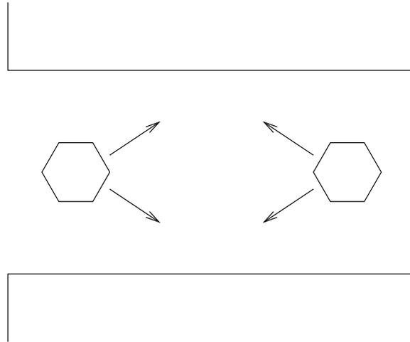
Figure 6: An illustration of the need for mixed strategies. The left robot attempts to pass through a corridor while the right robot attempts to block its progress. Each must independently decide whether to move to the left or right. If the left robot plays a pure strategy, the right robot can take advantage and always get in the way. A mixed strategy that chooses each direction equally often will enable the left robot to escape.
