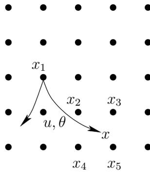
Figure 5: Dots denote sample states. Applying an action  $u$  and nature action  $\theta$  on a sampled state  $x_1$  moves the system to state  $x$  which is not in the sampled set. Some form of interpolation is needed to estimate the value function at  $x$ .
