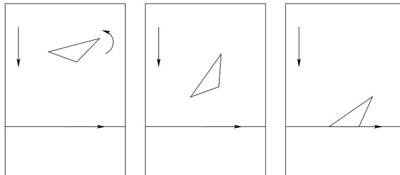
Figure 8: Overhead overview of a part on the conveyor. The conveyor moves downward. The robot picks up a part and rotates it through a chosen angle before placing it on the conveyor. The part then drifts on the conveyor into contact with the fence, possibly rotating compliantly as it comes to rest.
