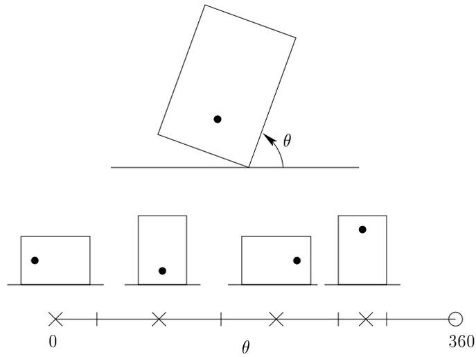
Figure 9: Effects of rotation actions on a rectangular part. The action space is divided into four equivalence classes according to the resulting state. The crosses mark a representative action from each class.
