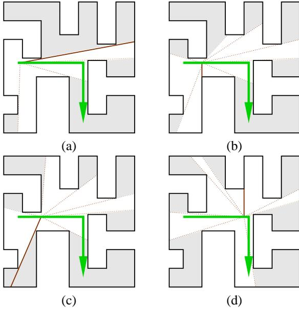
Fig. 3. In this simple example, a single robot carries a standard visibility sensor in a polygonal free space. The segment that emanates from the robot trajectory indicates where a component event occurs (only a few component events are shown). Agent trajectories are not shown. There are four possible types of component events: a) A shadow component *splits* into two. b) A shadow component *appears*. c) Two shadow components *merge*. d) A shadow component *disappears*.
